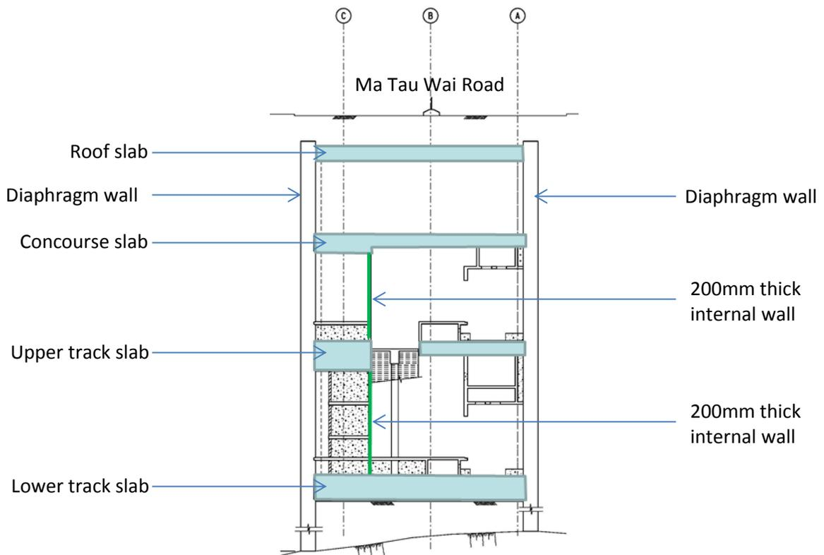
Figure 1 – Typical Cross section of To Kwa Wan Station
