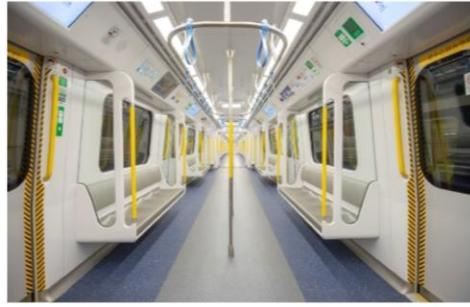
Train bodies are about 12cm wider than that of the existing trains, providing a more spacious travelling environment and narrowing the platform gap
